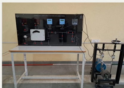
CONTROL PANEL FOR TO STUDY LOAD TEST OF DC SERIES MOTOR
