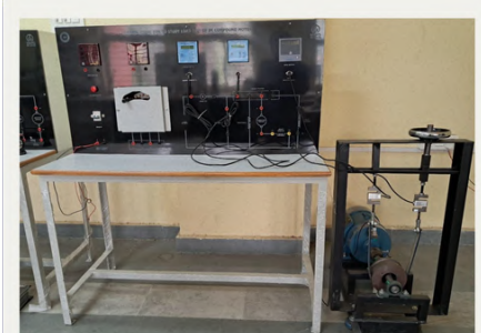
CONTROL PANEL FOR TO STUDY LOAD TEST OF DC COMPOUND MOTOR
