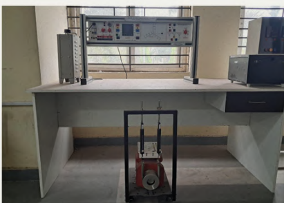
SINGLE PHASE AC INDUCTION MOTOR TRAINER
