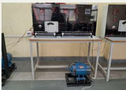
CONTROL PANEL FOR SWINBURN TEST AND SPEED CONTROL OF DC SHUNT MOTOR
