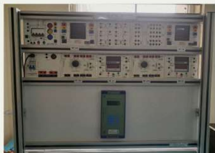
EXPERIMENTAL SETUP FOR PERCENTAGE BIASED DIFFERENTLY RELAY TESTING KIT.
