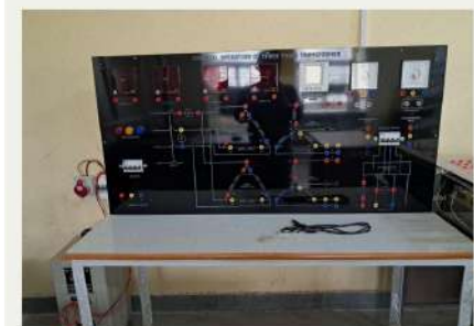
PARALLEL OPERATION OF THREE PHASE TRANSFORMER
