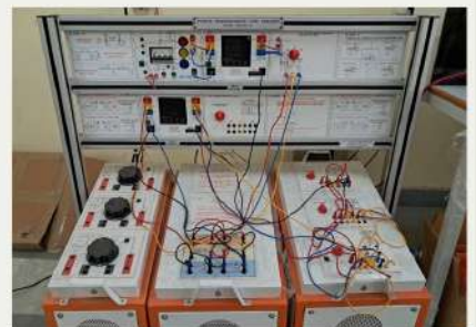
POWER TREANSMISSION LINE TRAINER
