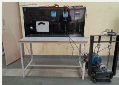
CONTROL PANEL FOR TO STUDY LOAD TEST OF SHUNT MOTOR
