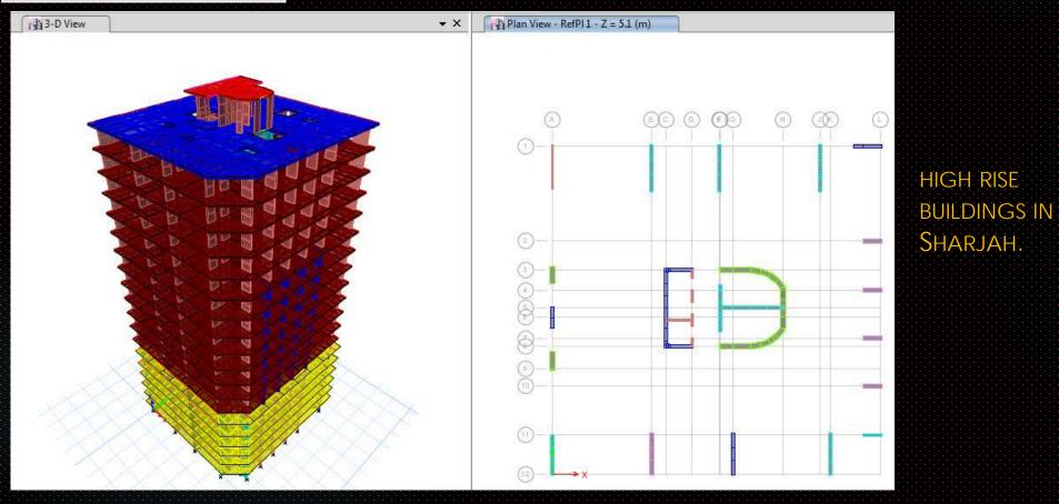
A SAMPLE OF ONE G+5P+13 TYP. FLOORS BUILDING WITH SHEAR WALL AND CENTRAL CORE, DESIGNED BY ER. SHAHI.
