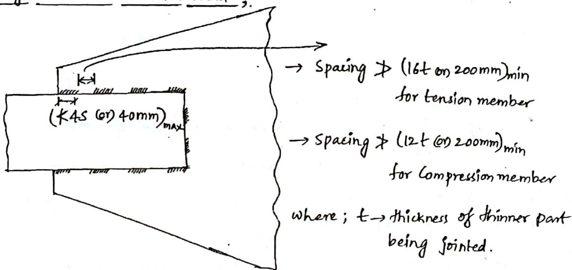
When the length of smallest size billet-weld required to transmit load is less than the continuous length of joint, intermittent fillet weld will be provided. But intermittent fillet weld cannot be used for dynamic & repetitive loads.
