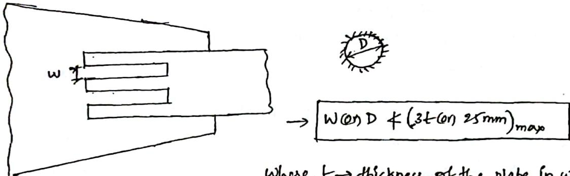
where,  $t \rightarrow$  thickness of the plate in which slot is made.
