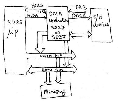
The Process of data transfer between the system memory and Peripheral under DMA controller can be classified between two mode.
