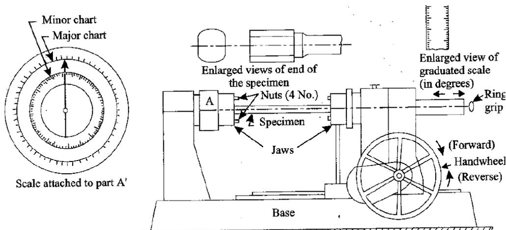
Fig:- Torsion Testing Machine
