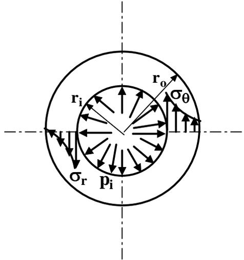
**9.2.1.3F- Radial and circumferential stress distribution within the cylinder wall when only internal pressure acts.**
