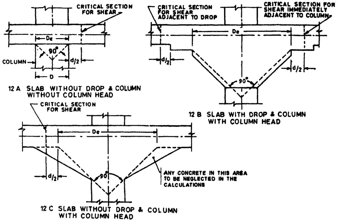
NOTE —  $D_c$  is the diameter of column or column head to be considered for design and  $d$  is effective depth of slab or drop as appropriate.
