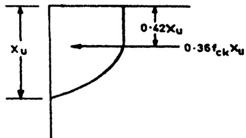
FIG. 22 STRESS BLOCK PARAMETERS
