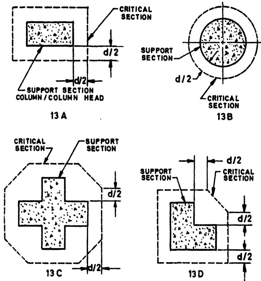
NOTE —  $d$  is the effective depth of the flat slab/drop.
