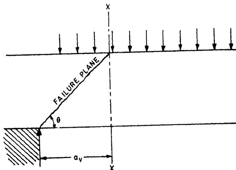
NOTE — The shear causing failure is that acting on section X-X.
