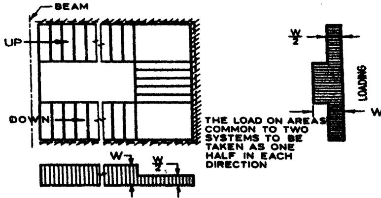
FIG. 18 LOADING ON STAIRS WITH OPEN WELLS
