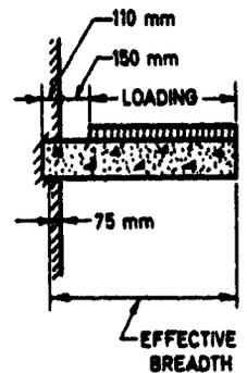
FIG. 19 LOADING ON STAIRS BUILT INTO WALLS
