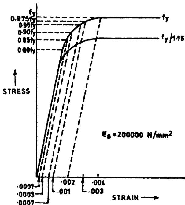
23A Cold Worked Deformed Bar
