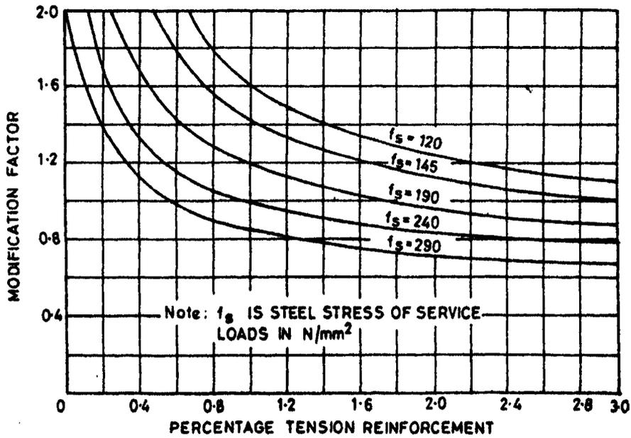
$$f_t = 0.58 f_s \frac{\text{Area of cross-section of steel required}}{\text{Area of cross-section of steel provided}}$$
