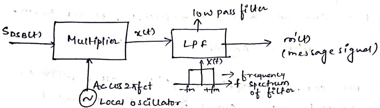
Here, DSB-SC signal is applied to multiplier or product modulator in which it is multiplied with the locally oscillator generated carrier.
