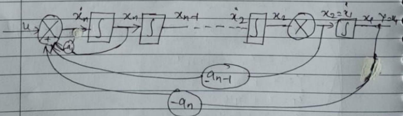
State Model of an nth order system in which the forcing function involves derivative terms.
