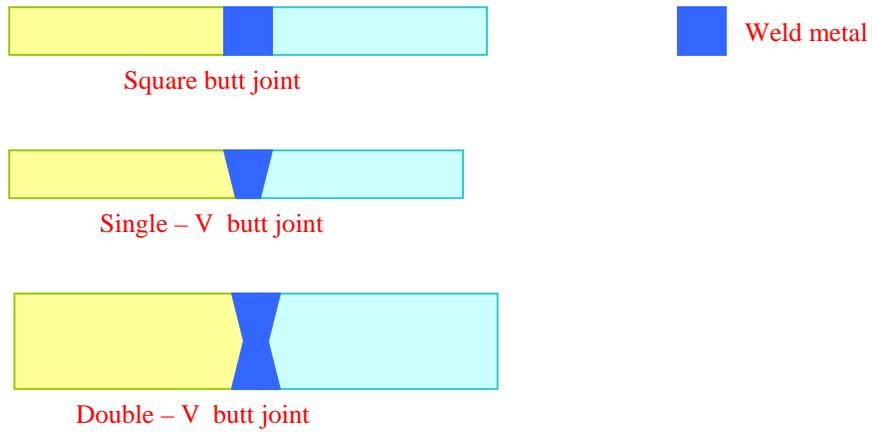
Figure 10.3.2: Different types of butt joints
