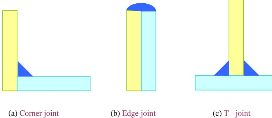
Figure 10.3.3: Other types of welded joints
