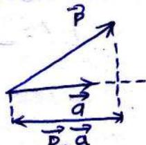
Hence the component of  $\vec{A}$  in the direction of  $\vec{a}_r$  is the dot product of  $\vec{A}$  with  $\vec{a}_r$ . This component is nothing but  $A_r$ .
