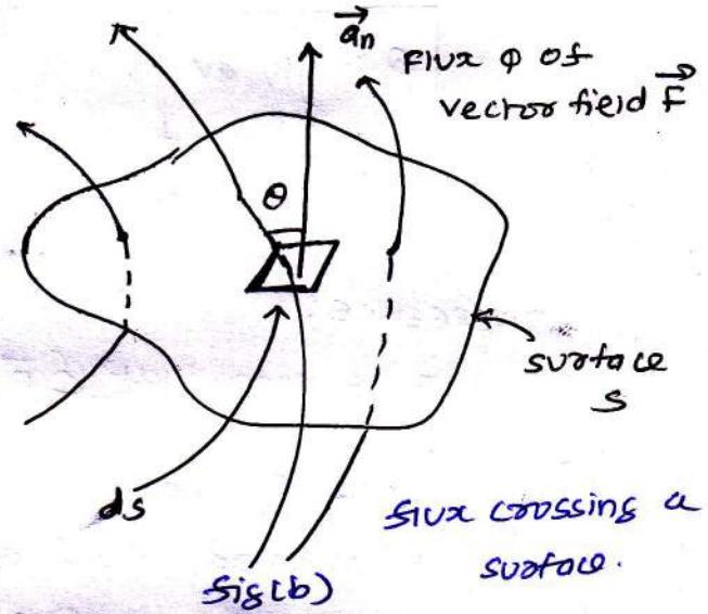
similarly a flux  $\phi$  may pass through a surface as shown in fig(b). While doing analysis of such cases an integral is required called SURFACE INTEGRAL, to be carried out over a surface related to a vector field.
