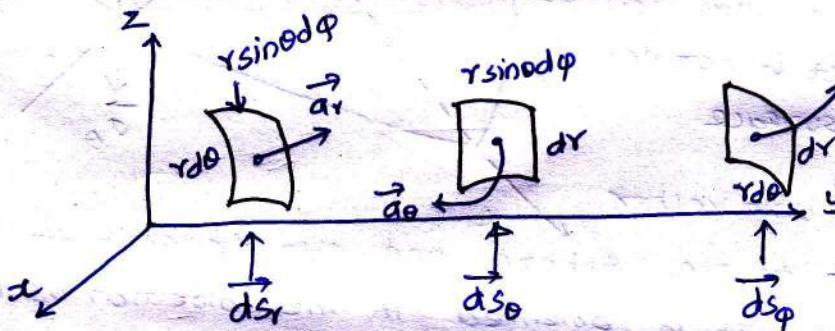
$$\vec{ds_r} = r^2 \sin\theta d\theta d\phi \quad \vec{ds_\theta} = r \sin\theta dr d\phi \quad \vec{ds_\phi} = r dr d\theta$$
