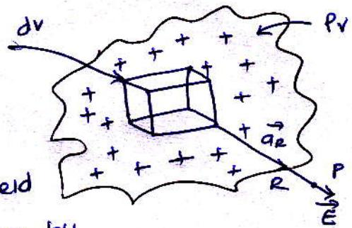
Hence the total  $\vec{E}$  at a point P is to be obtained by integrating  $\vec{dE}$  over the volume in which charge is accumulated. Note that this integration will be a triple integration.
