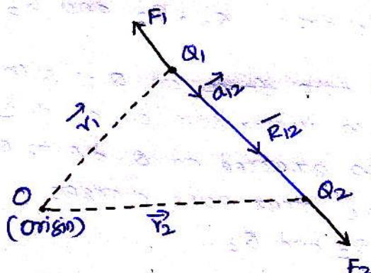
Then the force exerted by  $Q_1$  on  $Q_2$  acts along the direction  $\vec{R}_{12}$  where  $\vec{a}_{12}$  is unit vector along  $\vec{R}_{12}$ . Hence the force in the vector form can be expressed as.
