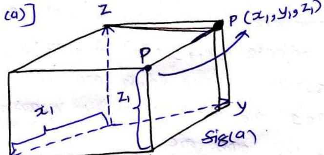
Consider a point  $P[x_1, y_1, z_1]$  in cartesian co-ordinate system as shown in fig (c). Then the position vector of point 'P' is represented by the distance of point P from the origin of point P from origin to point directed from origin to point P. This is also called RADIUS VECTOR.
