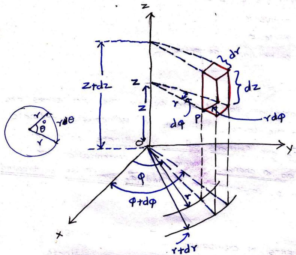
Hence the differential vector length in cylindrical co-ordinate system is given by,
