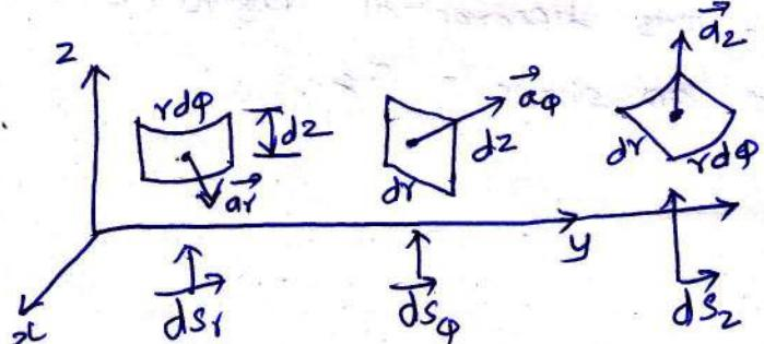
$$\begin{aligned}\vec{ds}_1 &= r d\phi dz \vec{a}_r \\ \vec{ds}_\phi &= dr dz \vec{a}_\phi \\ \vec{ds}_z &= r d\phi dr \vec{a}_z.\end{aligned}$$
