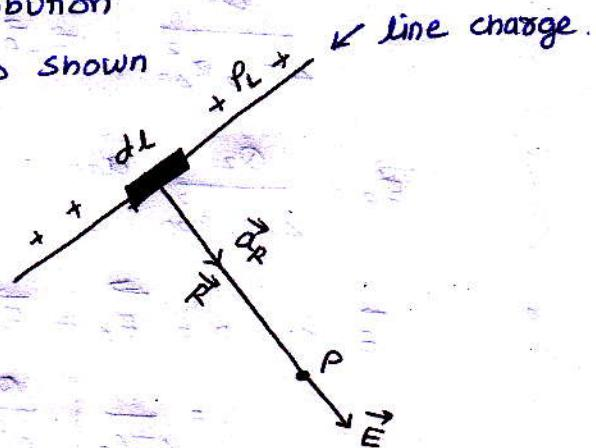
Hence the differential electric field  $\vec{dE}$  at point  $P$  due to  $dQ$  is given by.
