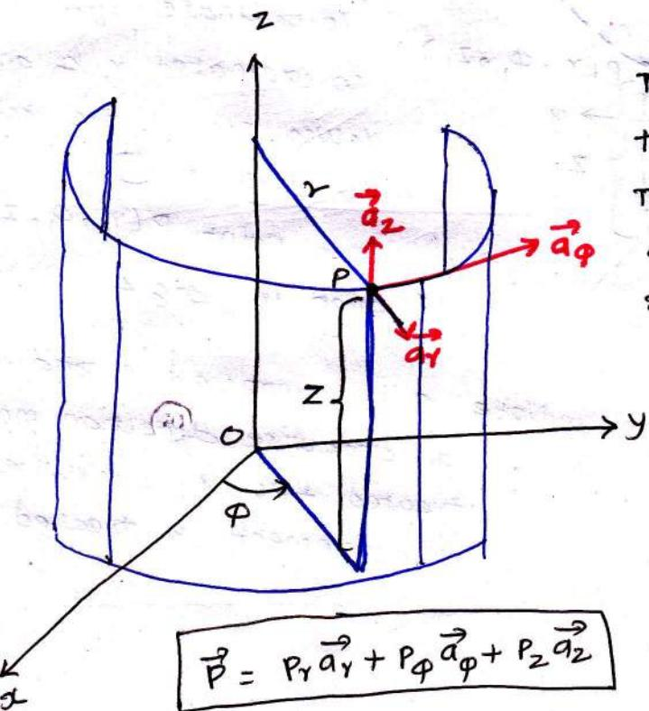
The  $\vec{a}_r$  lies in a plane  $\parallel^{el}$  to the  $xy$  plane and is  $\perp^r$  to the surface of the cylinder at a given point pointing radially outward.
