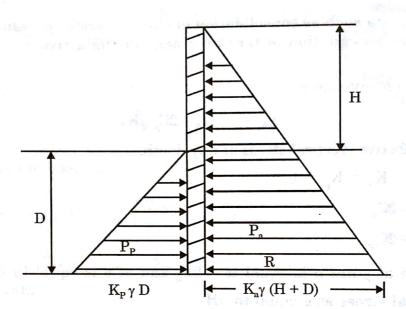
Let D be the depth of the embedment and H be the height of the cantilever sheet pile above the dredge level.
