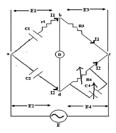
$$r_1R_4 - \{(jR_4)/(\omega C_1)\} = \{(-jR_3)/(\omega C_2)\} + \{(R_3R_4C_4)/(C_2)\}$$
