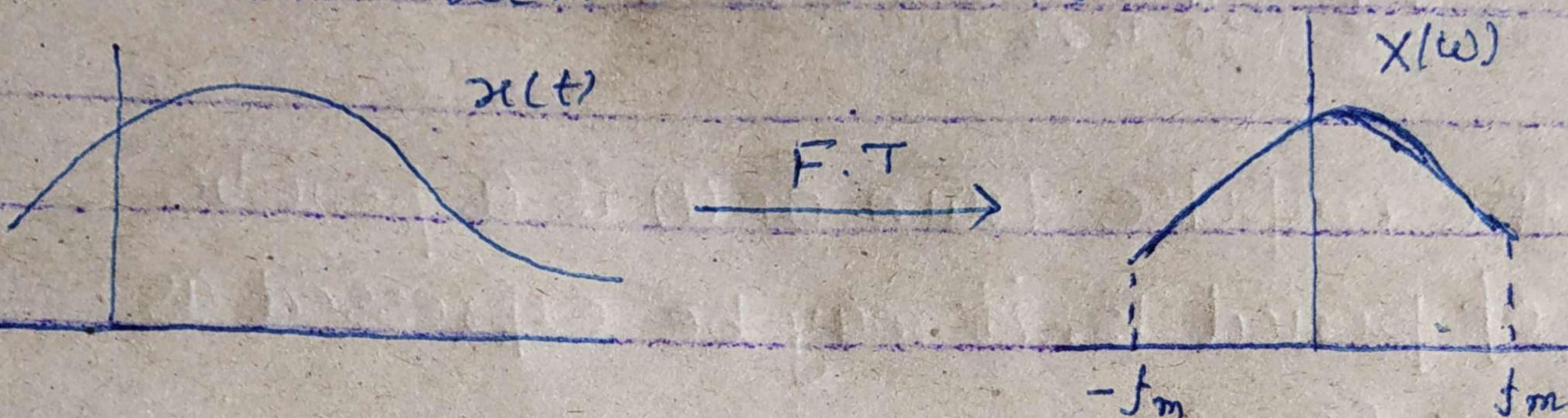
Sampling of  $x(t)$  at a rate of  $f_s$  Hz may be achieved by multiplying  $x(t)$  by an impulse train  $\delta_{T_s}(t)$ . The impulse train  $\delta_{T_s}(t)$  consists of unit impulses repeating periodically every  $T_s$  seconds, where  $T_s = \frac{1}{f_s}$ .
