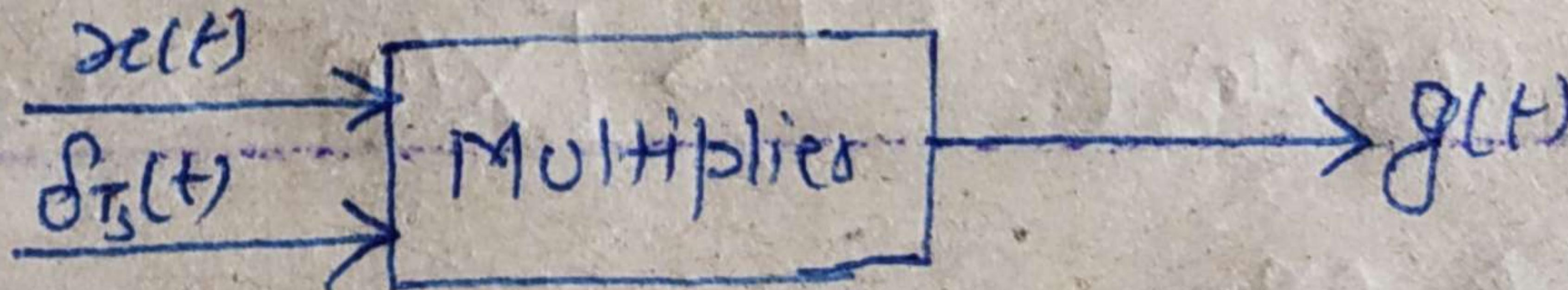
This sampled signal consists of impulses spaced every  $T_s$  seconds (the sampling interval). The resulting or sampled
