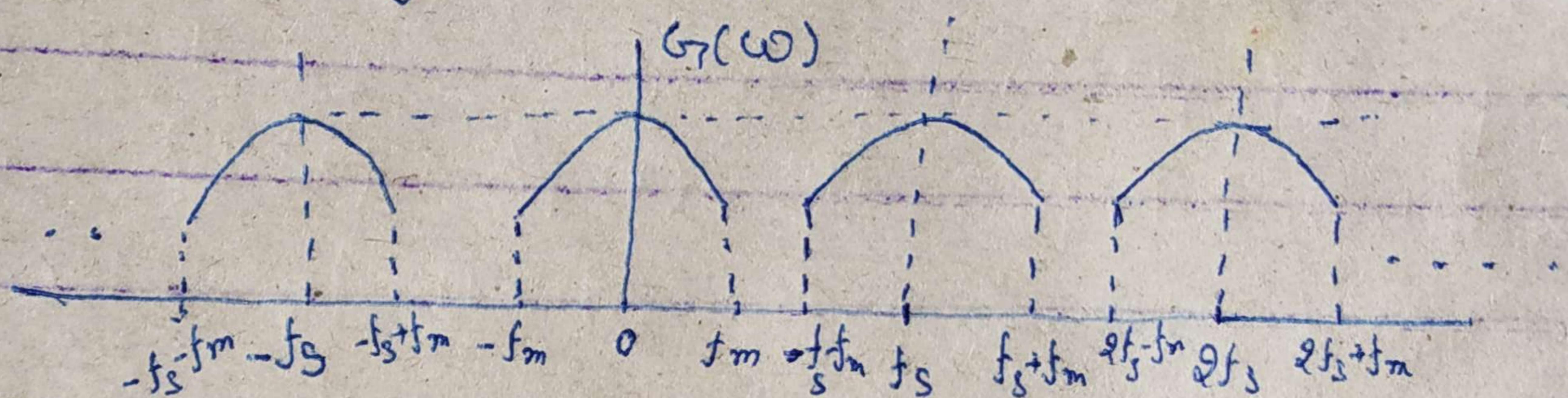
to reconstruct  $x(t)$  from  $g(t)$ , we must be able to recover  $X(\omega)$  from  $G_I(\omega)$ , this is possible there is no overlap between successive cycles of  $G_I(\omega)$ . This requires
