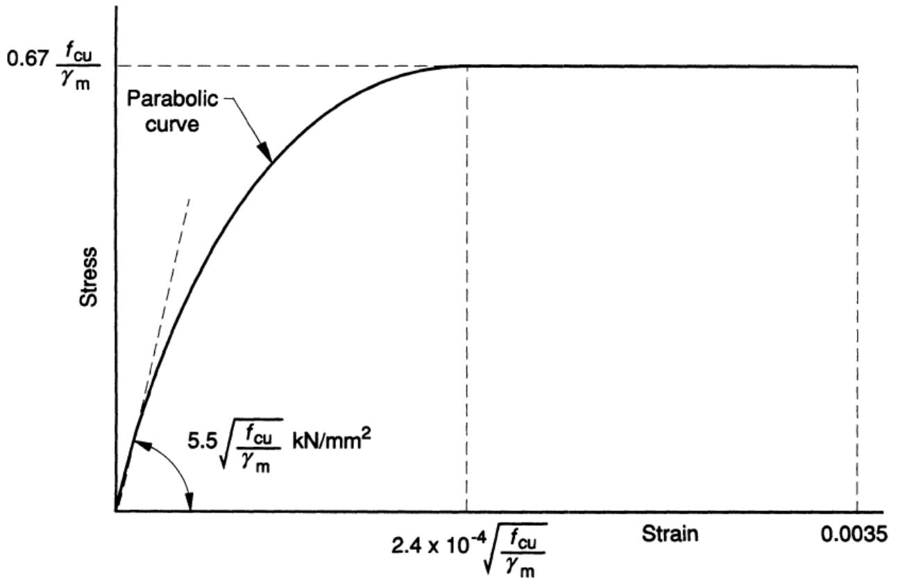
**Stress-Strain Curve for Concrete from BS8110**
