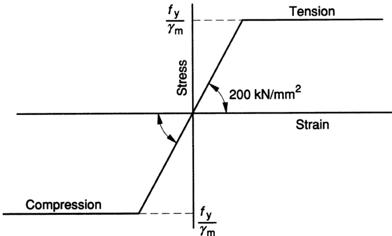
Stress-Strain Curve for Steel from BS8110
