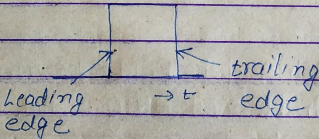
In other variation, the trailing edge is held constant and with respect to it pulse width is measured. In third variation, centre of the pulse is held constant and pulse width changes on either side of the centre of pulse.
