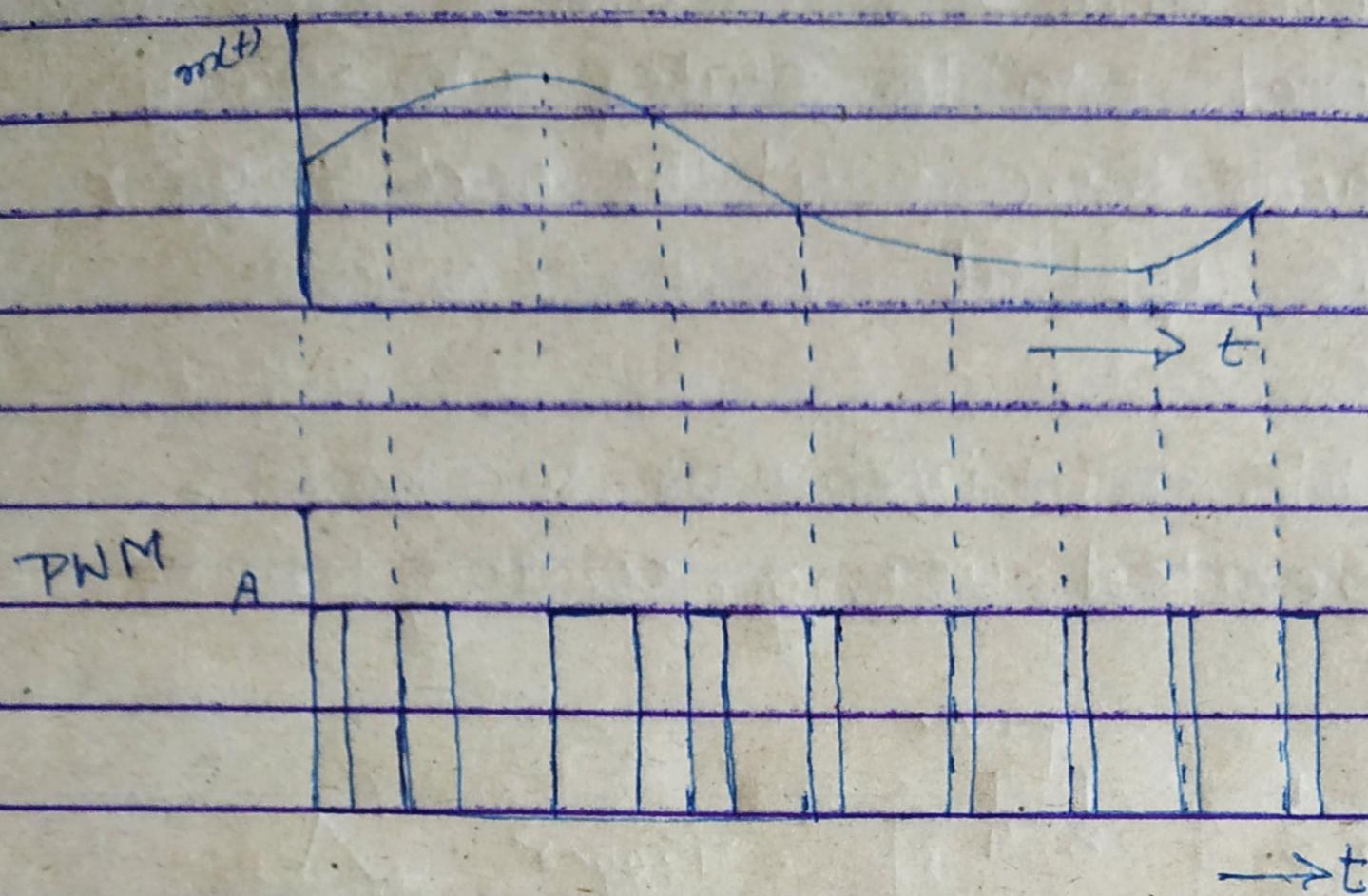
In the above diagram, the leading edge of pulse is held constant and the duration of pulse is varied in accordance with the instantaneous value of message signal  $m(t)$ .
