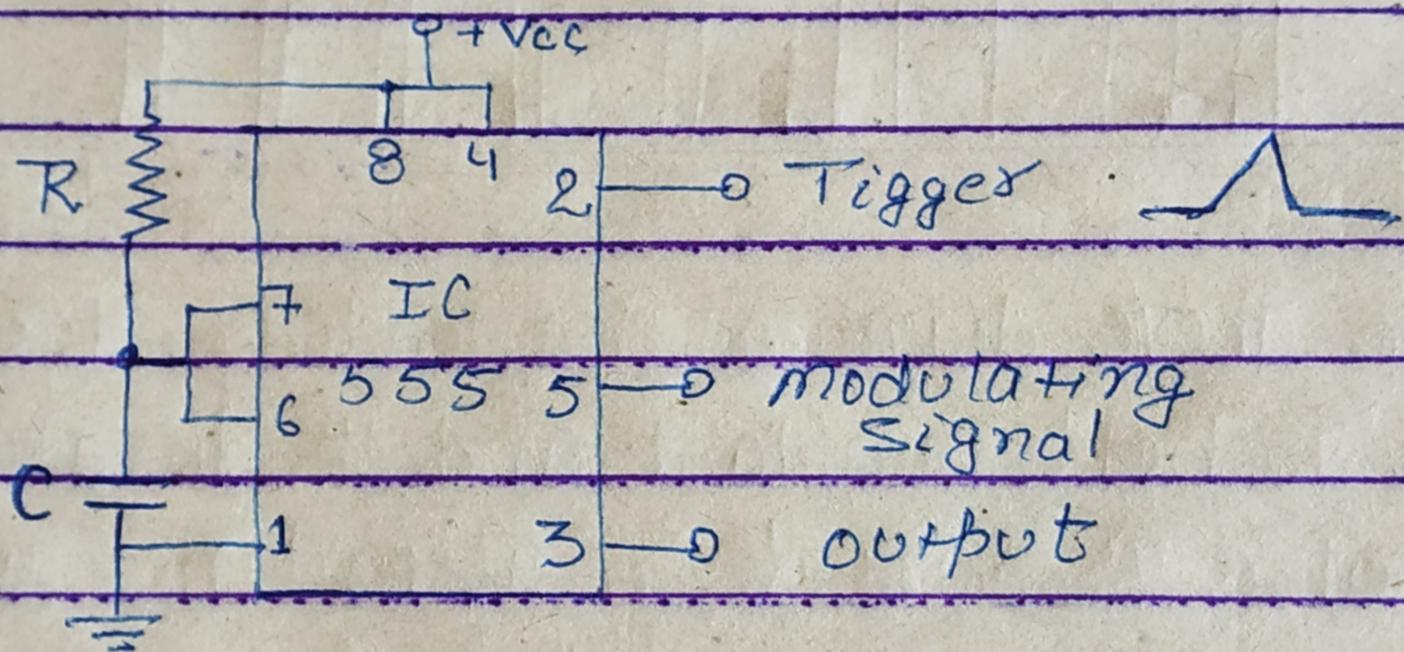
In monostable multivibrator, modulating input signal is applied at the control voltage input. Internally, the control voltage is adjusted to  $\frac{2}{3} V_{cc}$ . Externally applied modulating signal changes the control voltage and, hence the threshold voltage level. As a result, the time period required to charge the capacitor up to threshold voltage level changes, giving pulse modulated signal at the output.
