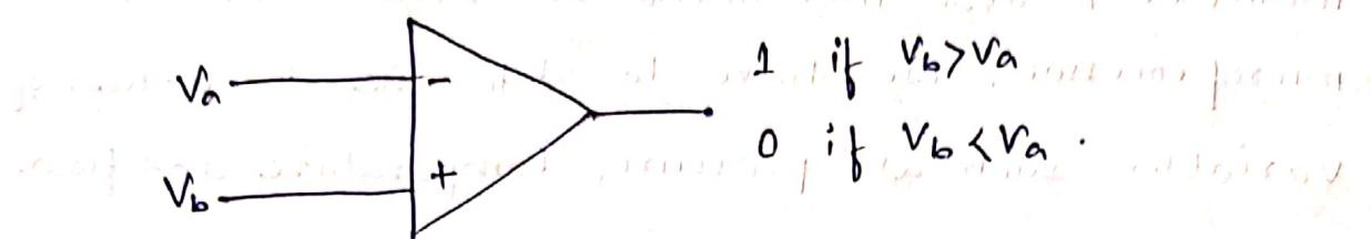
One of the voltages on the comparator i/p's,  $V_a$  or  $V_b$ , will be the variable i/p, and the other a fixed value called a trip, trigger or ~~ref~~ reference voltage.
