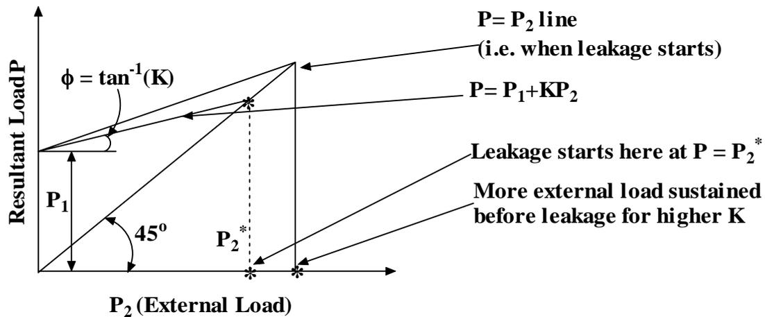
**4.4.3.1F** – Force diagram for joint separation
