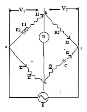
So,  $L_x = \frac{R_2 R_3 C_1}{1 + (\frac{1}{Q})^2}$ , but for high values of Q (i.e.) Q > 10 the term  $(\frac{1}{Q})^2$  is negligible.
