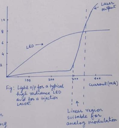
Signal transmission, direct analog signal are used for modulation of laser source. This means, laser source provides high signal to noise ratio (means high laser output), high end to end linearity to avoid any direct operation in phase and amplitude and crosstalk between multichannel signal transmission
