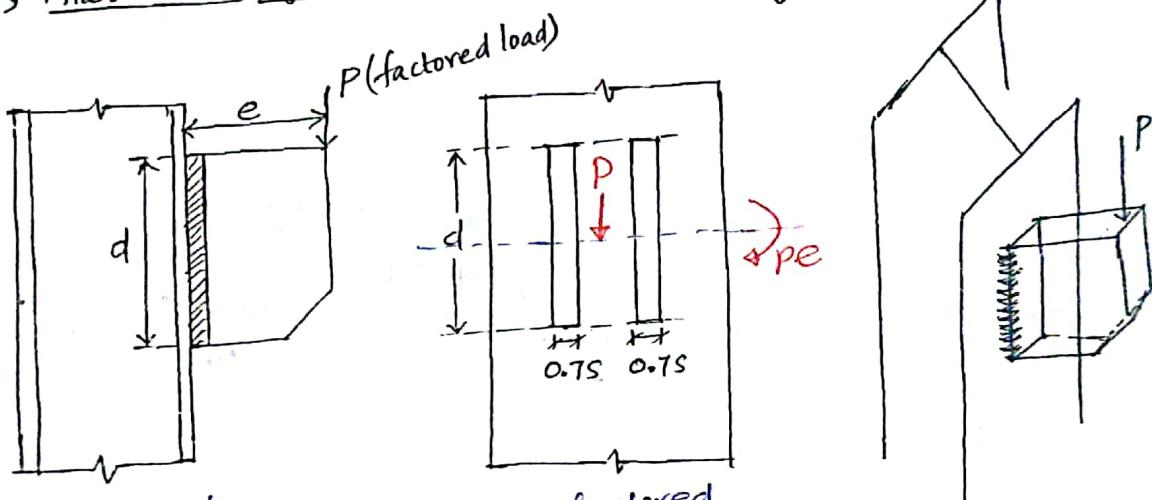
$q \rightarrow$  shear stress in weld due to load  $P$  ;  $q = \frac{P}{2d t_w}$
