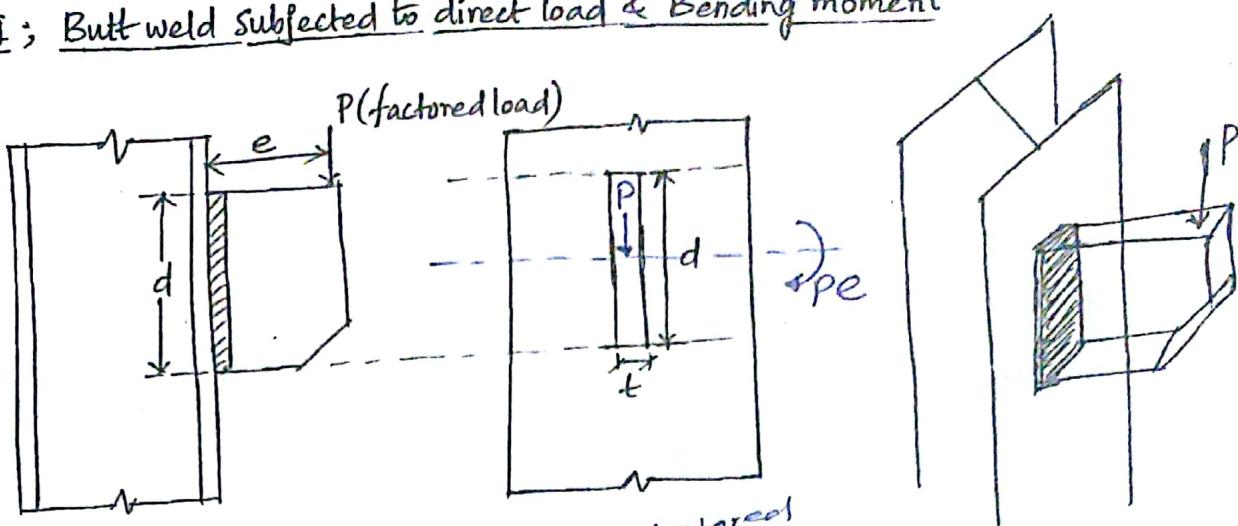
$q \rightarrow$  Shear stress on weld due to load  $P$
