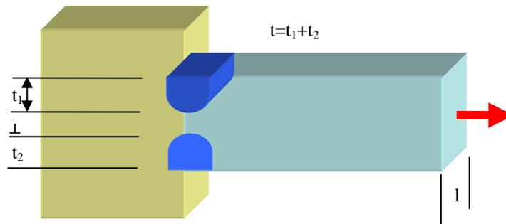
Figure 10.4.1: Design of a butt joint
