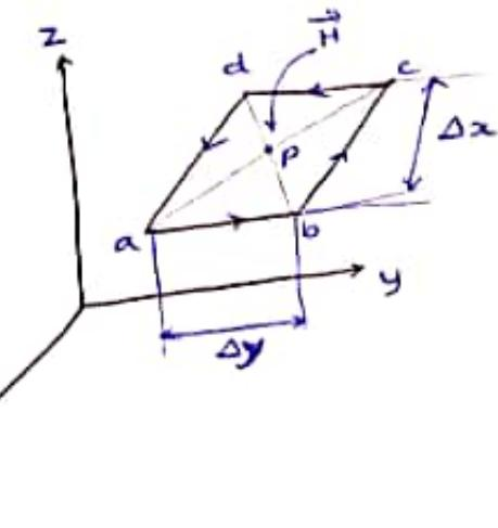
Now  $H_x$  can be expressed in terms of  $H_{x0}$  at Point P and rate of change of  $H_x$  in y direction and y.
