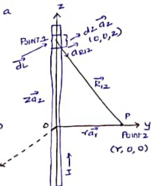
thus total flux intensity  $\vec{H}$  can be obtained by integrating  $d\vec{H}$  over the entire length of the conductor. (5)
