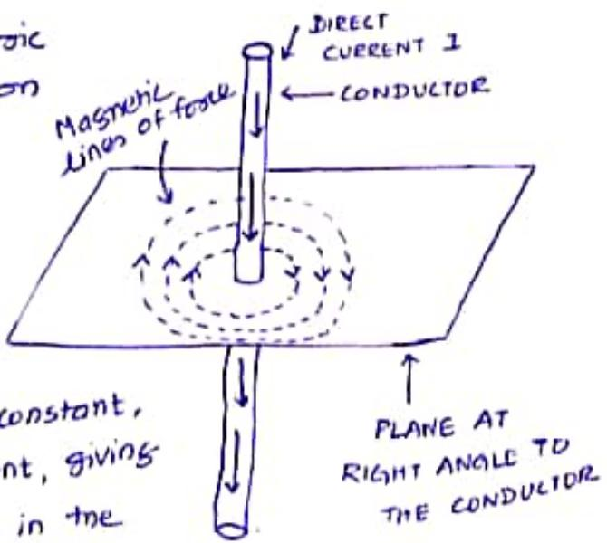
A right hand thumb rule is used to determine the direction of magnetic field around a conductor carrying a direct current. It states that, hold the current carrying conductor in right hand such that thumb pointing in the direction of current and  $\parallel$  to the conductor, then curled fingers point in the direction of the magnetic lines of flux around it.
