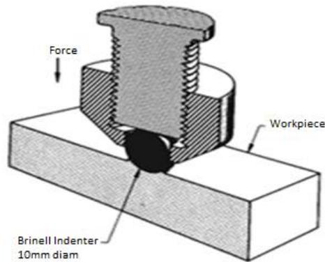
Compared to the other hardness test methods, the indenter used in Brinell makes the deepest and widest indentation, so that test averages the hardness over a wider amount of materials which will account for multiple grain structures and any irregularities in the uniformity of the material.
