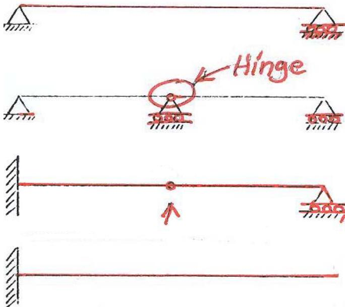
Consider the beam to the left. The beam is statically indeterminate to the second degree. A statically determinate structure can be obtained by releasing two redundant reactions. Four possible released structures are shown.
