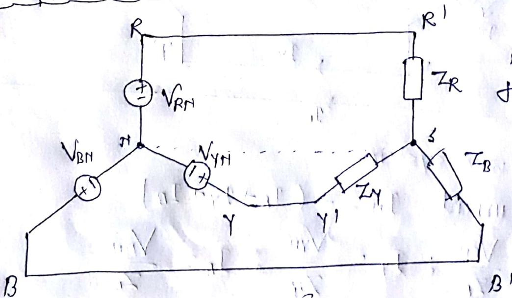
By applying Millman's theorem the above circuit can be simplified to
