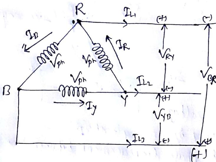
$$V_{RY} = V_{YB} = V_{BR} = V_L \quad \left\{ \begin{array}{l} I_{L1} = I_R - I_B; \\ I_{L2} = I_Y - I_R; \\ I_{L3} = I_B - I_Y; \end{array} \right.$$
